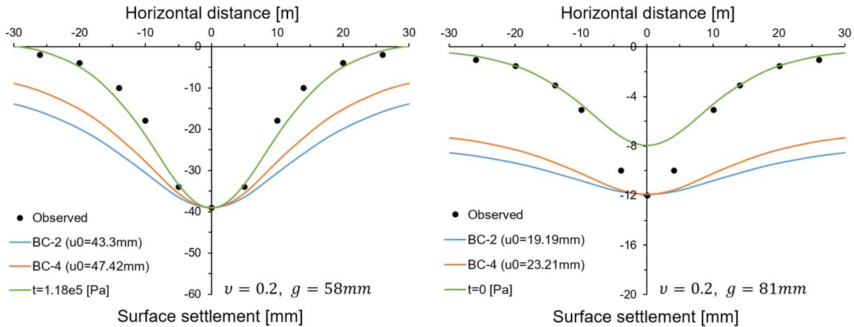
**Figure 2.** Observed and predicted surface settlement. (Left) Heathrow Express Trial Tunnel; (Right) Bangkok Sewer Tunnel.
